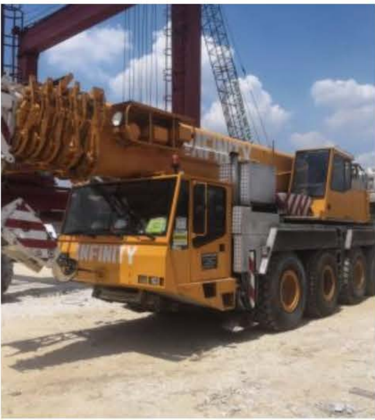
80T All Terrain Crane
